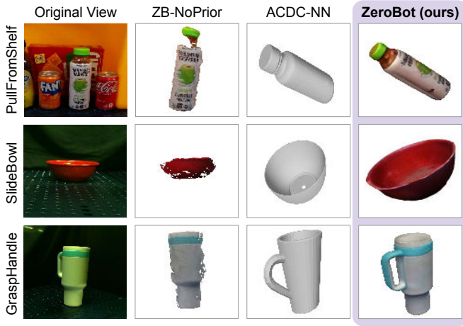
Fig. 7: Qualitative results comparing mesh generation methods. ZeroBot generates a mesh which is complete and more accurate than the baselines, improving sim2real success rates.
