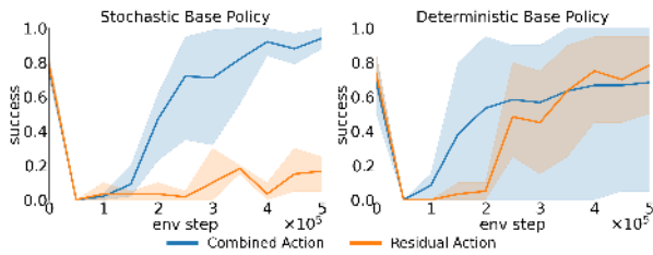
Fig. 5: Learning with either the residual or the complete action works well with deterministic base policies, but learning with complete action is required for stochastic base policies.
