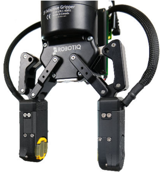
Fig. 1. Prototype fingertips with pivotable, brakeable rollers mounted on a Robotiq 2F-85 Adaptive Gripper.
