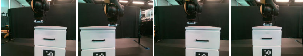
Figure 9: Samples from the initial state distribution of the collected demonstrations for the Spot drawer opening experiments. For this task, the factors of variation are the position and orientation of the robot with respect to the drawer.
